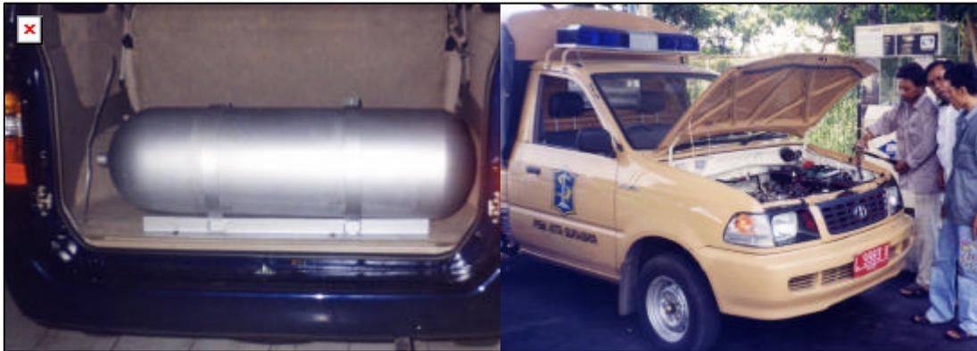
Right: The CNG tank in the back seat.
