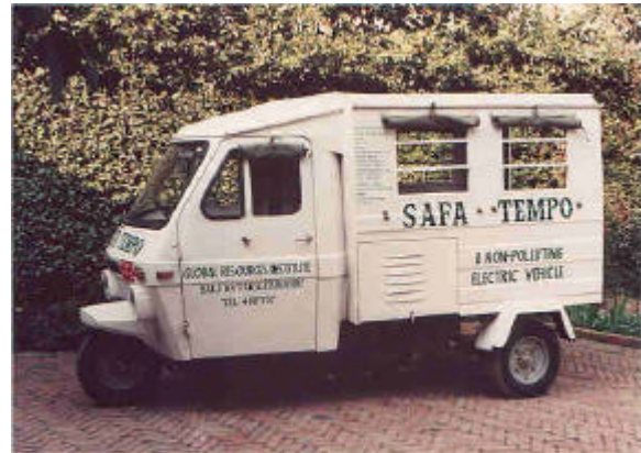
Figure 1. A typical battery operated three-wheeler in Kathmandu Valley (Courtesy: Clean Energy Nepal (CEN), Kathmandu, Nepal)
