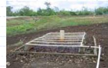
Circulation column with trickling filter
